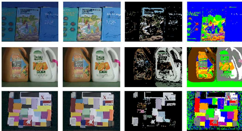
Figure 3.5: Controlled indoor dataset. Original image (left), corrected image by proposed method (center-left), points weighting the selected illuminant (center-right), categorisation of corrected images (right)
