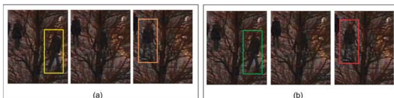
Figure 3.7 Problems with totally occluded objects. (a) The detection output across three adjacent frames. (b) The tracking performed without considering the object history; in this case a tracking algorithm would see the blob 2 as a new object in the scene, since in the previous frame there was no corresponding object.
