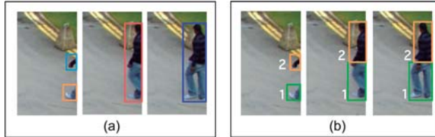
Figure 3.6 Problems with entering objects. (a) Blobs across three adjacent frames. (b) The tracking performed without considering the object history; in this case a tracking algorithm would not be able to distinguish this situation from two separate objects joining a group, and so attempts to preserve the separate identities of the two objects 1 and 2.
