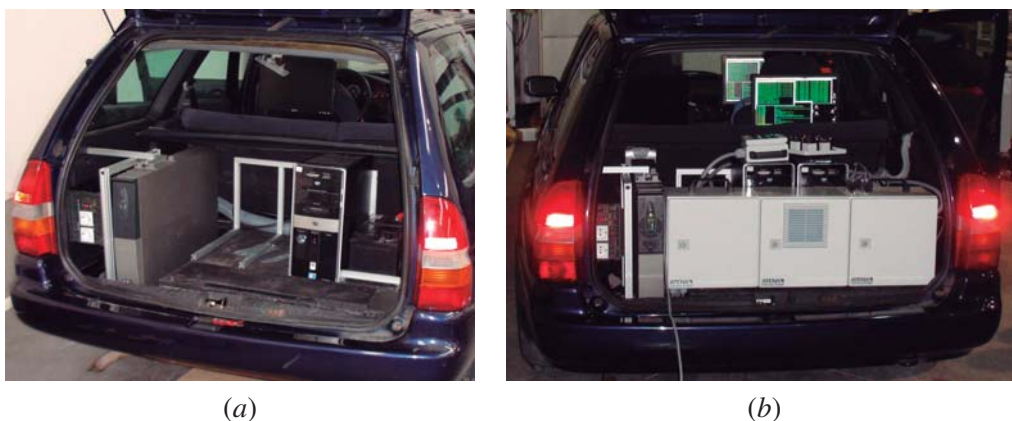
Figure 3.15: (a) The power stabilization equipment onboard the AtlasCar : from left to right, the inverter, the UPS, the buffer battery; (b) The final installation of the AtlasCar trunk. Inside the white boxes are the AC-DC power converters and the PLC.
