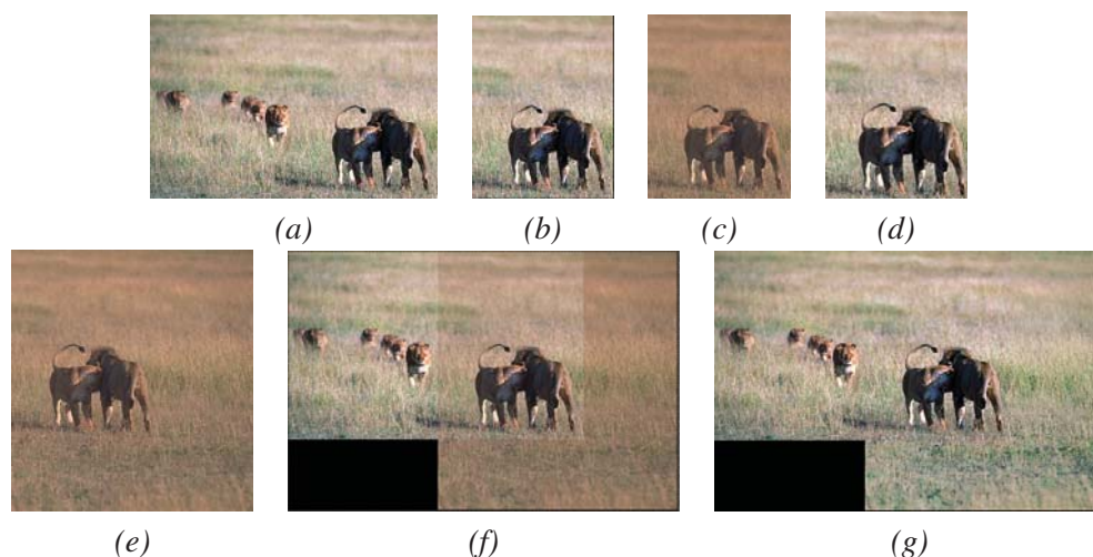
Figure 6.1: Images involved in a color correction procedure: (a) source image ( \mathbf{S} ); (b) overlapping area of the source ( \mathbf{S}_p ); (c) overlapping area of the target ( \mathbf{T}_p ); (d) overlapping area of the corrected image ( \hat{\mathbf{T}}_p ); (e) the target image ( \mathbf{T} ); (f) mosaic of source and target; (g) mosaic composed of the source and corrected images.
