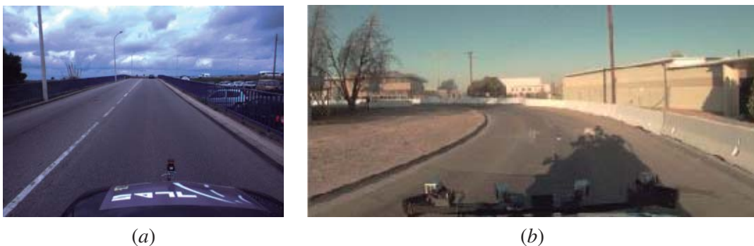
Figure 10.7: Images from onboard cameras sometimes view portions of the host vehicles: (a) AtlasCar stereo camera; (b) Talos forward center camera.
