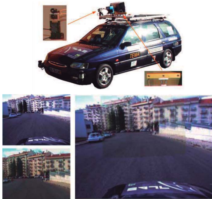
Figure 6.12: The AtlasCar robotic platform with several onboard cameras (top). Onboard images taken with two cameras from a typical road scene. Source image (bottom-left-top), Target image (bottom-left-bottom); the mosaic of both which shows a clear difference in colors (bottom-right); .
