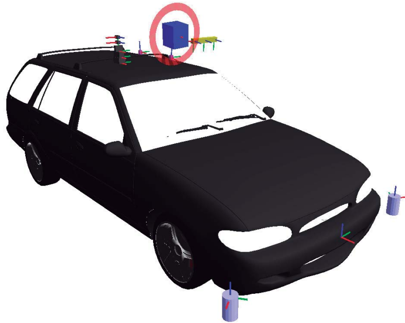
Figure 4.5: A 3D model of the AtlasCar and its onboard sensors visualised using RVIZ and the AtlasCar URDF . An interactive marker (red circle) enables the user to set the desired laser position.
