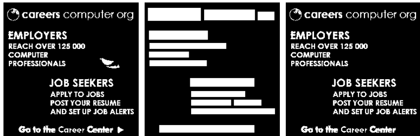
Figure: CC's before grouping. After grouping, each group is replaced by a white mask; thirteen distinct groups can be seen. Most of the non-text components are removed due to the overlap, which does not happen for the text components.
