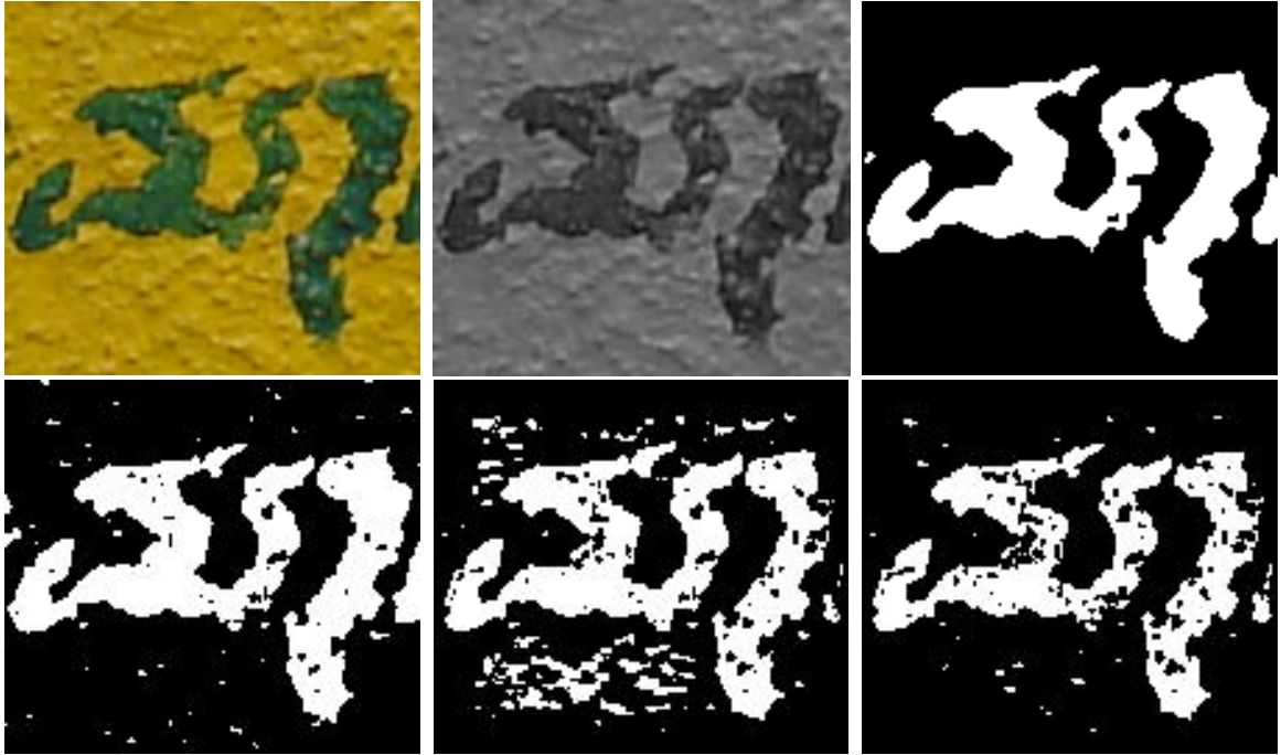
Figure 4.5: Comparison of outputs of different binarization techniques. (a) A sample image. (b) Gray scale image. (c) Classification of pixels using energy minimization function (MAPS). (d) Otsu's global thresholding. (e) Niblack's local thresholding. (f) Sauvola and Pietäikinen's local thresholding.
