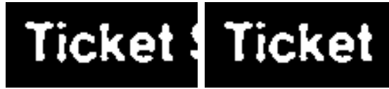
Figure 3.14: Removal of non-text components touching the boundary from born-digital images. Segmentation of a sample word image from born-digital 2011 data set using PLT. Few non-text components (the characters of neighboring words) appear as broken along the boundary.
