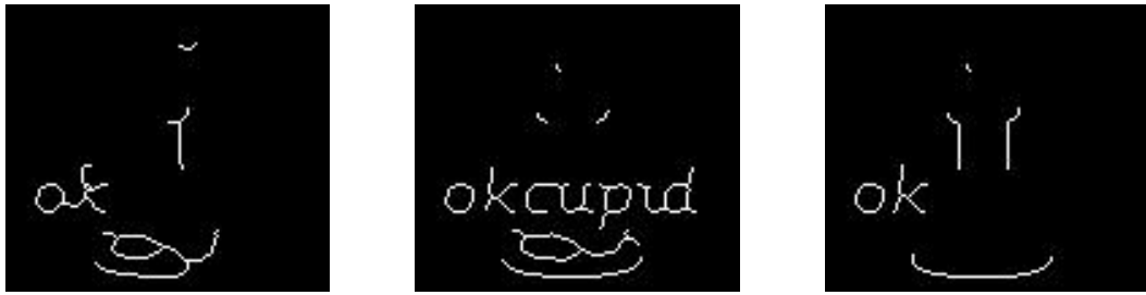
Figure 2.6: Thinned planes obtained after the merging operation in second section, where the text and non-text components are easily identified. (a) Thinned red plane ( I_{tr} ). (b) Thinned green plane ( I_{tg} ). (c) Thinned blue plane ( I_{tb} ).
