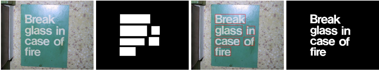
Figure 1.3: Illustration of the distinction between text localization and segmentation tasks. (a) A sample scene image from ICDAR 2003 data set. (b) Text localization mask. (c) Red coloured bounding box placed around each word. (d) Segmented text.
