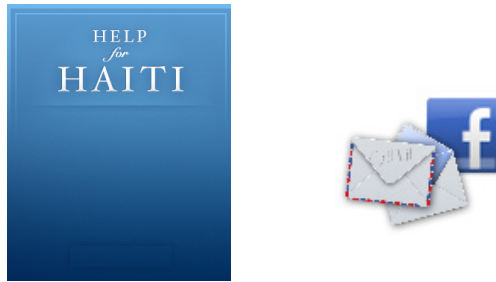
Figure 2.17: Images from the born-digital competition data set, where OTCYMIST method fails. The first image has low contrast. The second image has a single character, which gets eliminated during the grouping process, in the proposed method.
