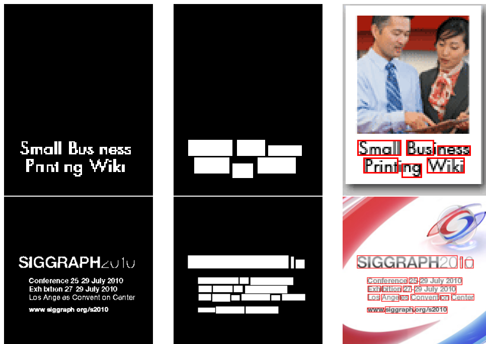
Figure 2.13: Segmented text, localized text and localized bounding box mask obtained by OTCYMIST method for test images from the born-digital data set.
