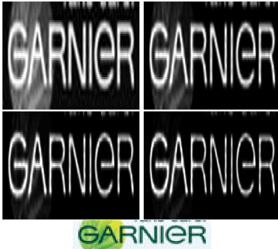
Figure 3.4: Contrast enhancement after power-law transformation with \gamma = 1, 2, 3 and 4 , respectively. The gray patch behind the letters ‘G’ and ‘A’ gradually decreases and becomes invisible for \gamma = 4 . Bottom row: Original image is shown for comparison.
