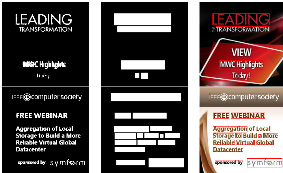
Figure 2.14: Segmented text, localized text and localized bounding box mask obtained by OTCYMIST method for test images from the born-digital data set.
