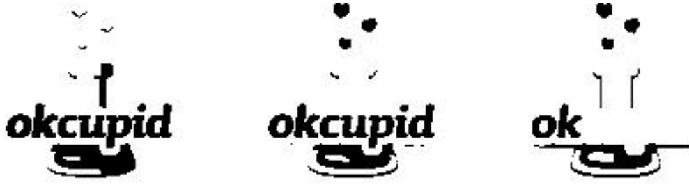
Figure 2.3: Results of Otsu's binarization of colour channels for the first image in Fig. 2.1. (a) Binarized red plane ( I_{br} ). (b) Binarized green plane ( I_{bg} ). (c) Binarized blue plane ( I_{bb} ).
