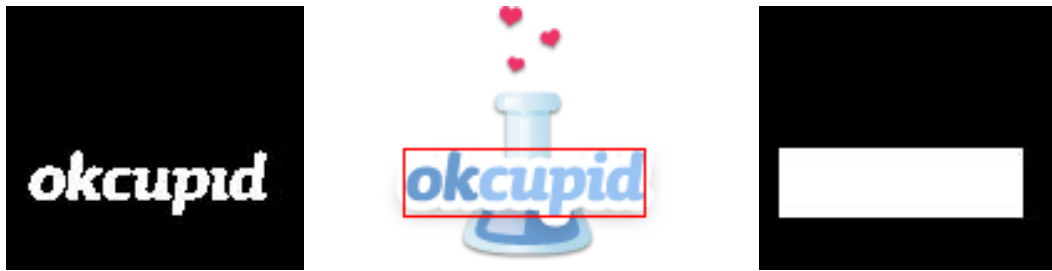
Figure 2.11: Result of the proposed OTCYMIST method for the first born-digital image in Fig. 2.1. (a) Segmented text. (b) Localized text. (c) Text Localization mask.
