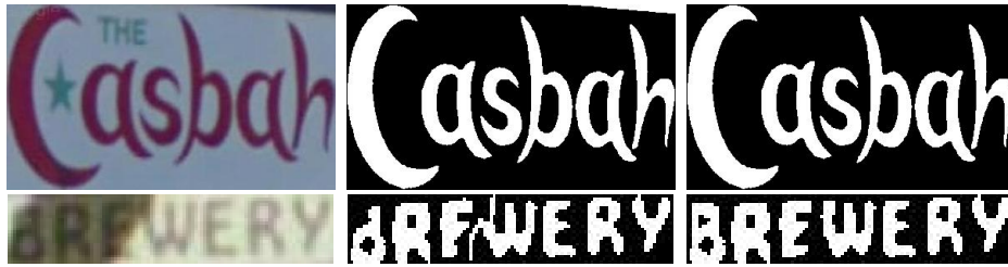
Figure A.4: Use of polygons to refine the best automated segmentation result. (a) Two sample word images from SVT dataset. (b) The segmentation results chosen by an user. (c) Segmented images after refinement by deletion and/or inclusion of appropriate regions defined using polygons.
