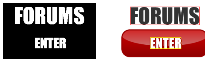
Figure 2.12: Segmentation and localization results of OTCYMIST method on the second image in Fig. 2.1, which has text of both polarities.
