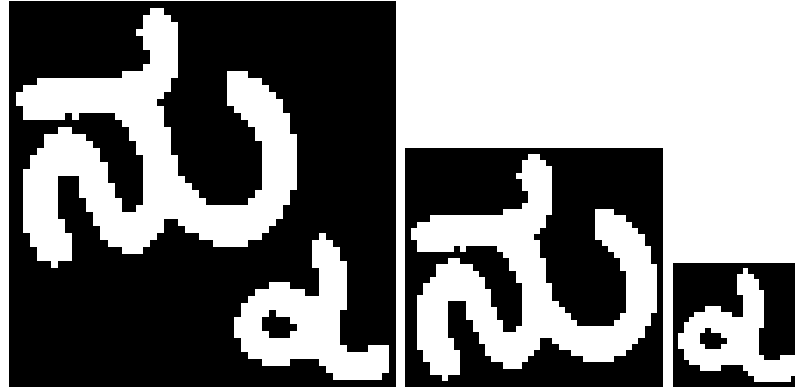
Figure 4.9: The segmented image has a base and a ottu component. The split occurred between the base and ottu components due to low overlap. The base and other components are shown in the middle and last columns, respectively.
