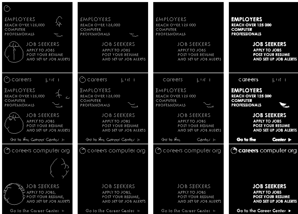
Figure 2.8: Analysis of minimum spanning tree on thinned colour planes. First column: Thinned colour channels for the last image in Fig. 2.1. Second column: Results after the first pass of minimum spanning tree. A few non-text components are removed. Third column: Results after the second pass of minimum spanning tree. Non-text components, which were still present, have now been removed. Fourth column: Connected components retrieved after the second pass of minimum spanning tree in each plane before merging into a single plane.
