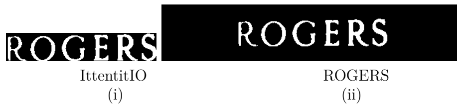
Figure 3.13: Post-processing the segmented image by padding background pixels to eliminate foreground-background ambiguity. (i) The text connected components touch the boundary. (ii) Foreground and background are clearly separated after background padding, leading to improved OCR results.
