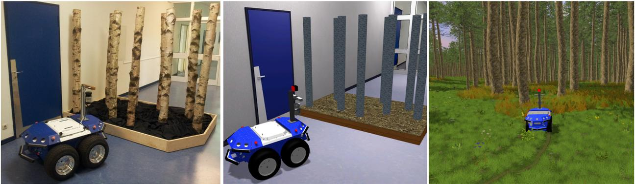
Figure 8: Left: Real test environment under laboratory conditions. Middle: Common virtual testing environment for testing of computer vision algorithms. Right: Close-to-reality virtual test environment using dynamic ground vegetation for more accurate testing results.
