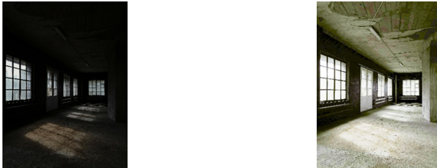
Figure 3: Comparison of RGB images from the graph in Fig 2 before (left side) and after (right side) histogram equalization
