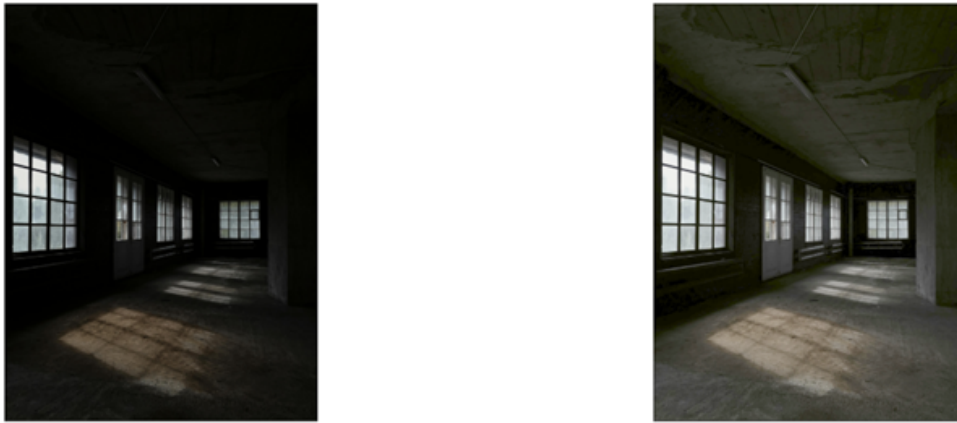
Figure 7: Comparison of RGB images from the graph in Fig 7 before (left) and after (right) gamma correction with \gamma = 0.5
