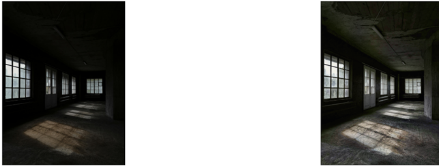
Figure 5: Comparison of RGB images from the graph in Fig 4 before (left) and after (right) CLAHE with clip limit of 3 and tile grid size of 8 x 8
