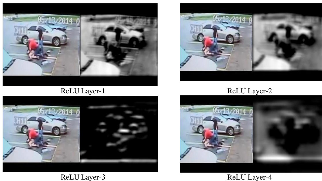
Figure 5 The largest activation at each ReLU layer for the arrest event
